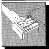
Pour the washing powder into compartment  $\ensuremath{\bigsqcup}$ , the main wash compartment.
